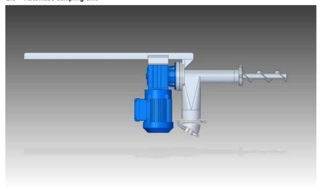
In the dosing hopper a sampling unit will be placed. A small screw will takes some product out of the hopper. This product will be dropped into a plastic sampling bag. In the display of the filling machine the operator chooses in what frequency the samples has to be taken. The screw and motor are easy to pull back via the guiding. This makes it easy to clean.
