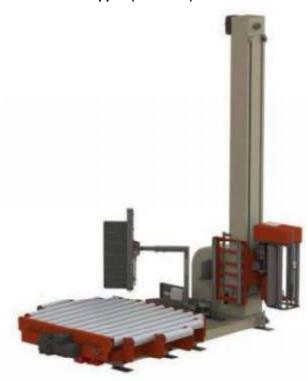
Fully automatic pallet-stretch wrapper. The pallet is turned around by a turning table.
