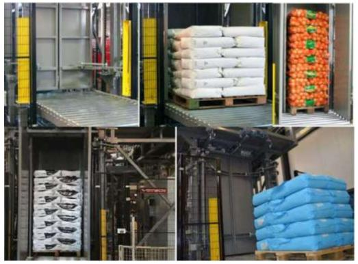
The lifting conveyor is placed in a shaft. Displays the pallet stacked. The box is adjustable for 4 modes. Once the pallet is ready the doors will open and run the full pallet and an empty pallet entered.
