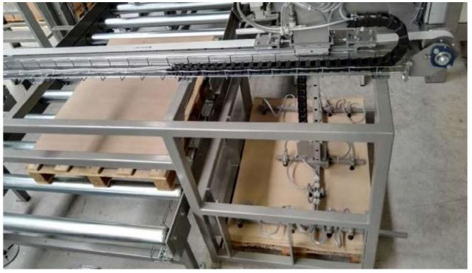
To place cardboard sheets onto the pallet. The sheetdispenser is able to move vertical and horizontal. The sheets can be placed into the sheetdispenser at a previous fixed position. Than the sheet is picked up by suction pads. When different sizes of sheets have to be produces it is possible to ajdust the suction pads.
